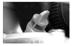
Engine oil filling cap and oil dipstick
